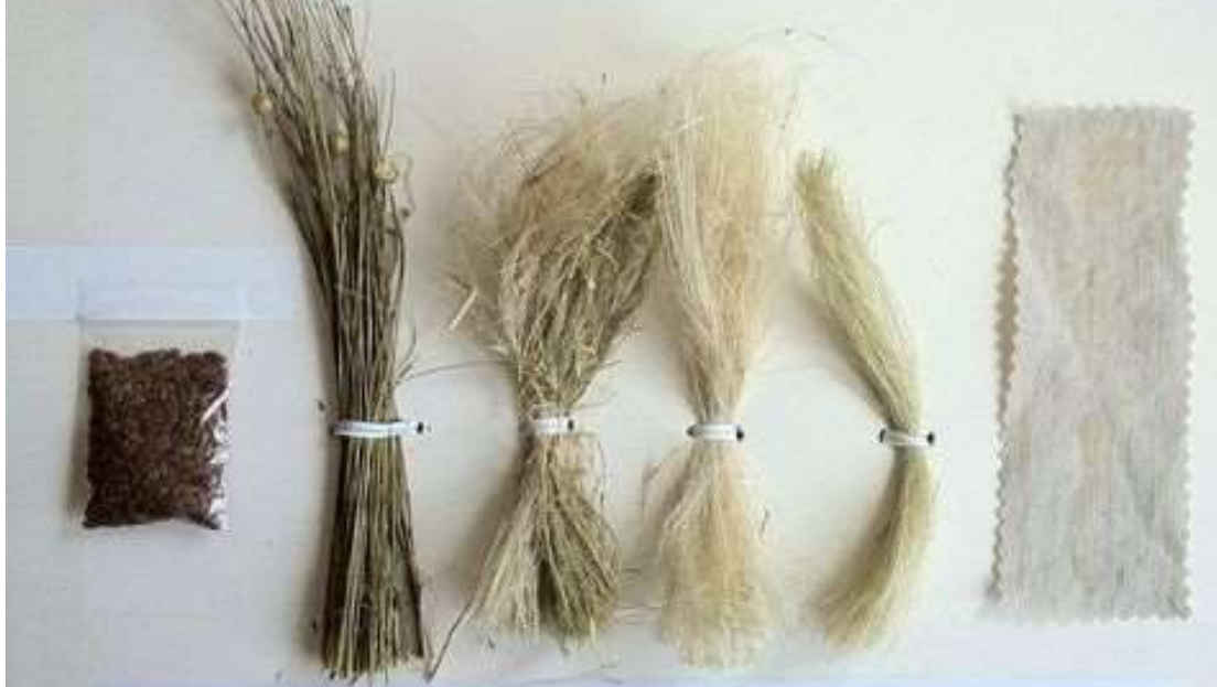
Flax seeds Green flax straw with seed pods Broken flax Scutched flax Combed flax Linen fabric
