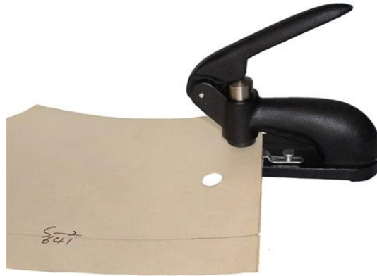
Figure 1.38 How to use a pattern punch
