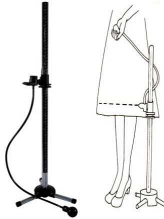
Figure 1.53 Skirt marker and method of use
