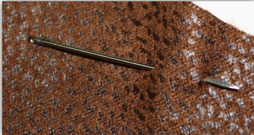
Figure 1.18 Needle used for leather work
